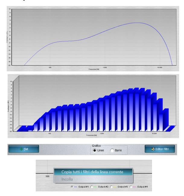
From this section it is possible to display the equalization curve of the various outputs; by clicking on the name of an output, the relevant equalization curve is displayed.
