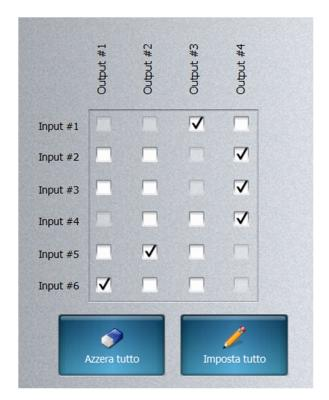
From this section it is possible to direct one or more input to one or more output by selecting the intersections of the bypass matrix "by putting a check mark".
