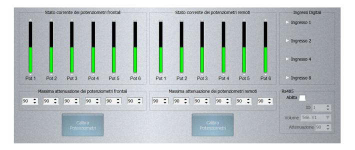
From this section it is possible to adjust the intervention level of each potentiometer both internal (front) and external (remote).
