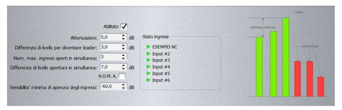
To activate the automatic control of the inputs, check the box "Abilitato".
