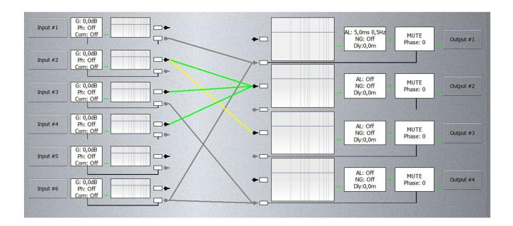
From this section it possible to control the flow of signals between inputs and outputs to get a global vision "at a glance"
