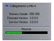
Monitor for connection status (ON-LINE o OFF-LINE), serial, service version (software running on PC), firmware (of the device) and total DSP resources
