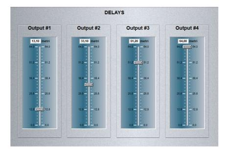
From this section it is possible to enable a delay for each output.
