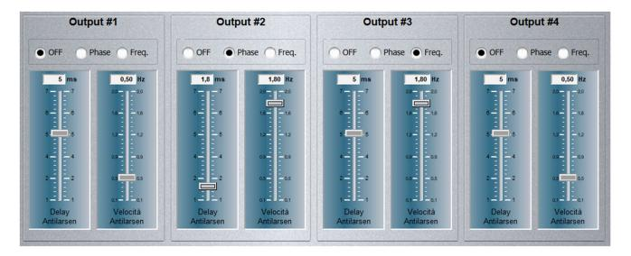
From this section it is possible to enable an antilarsen for each output.
