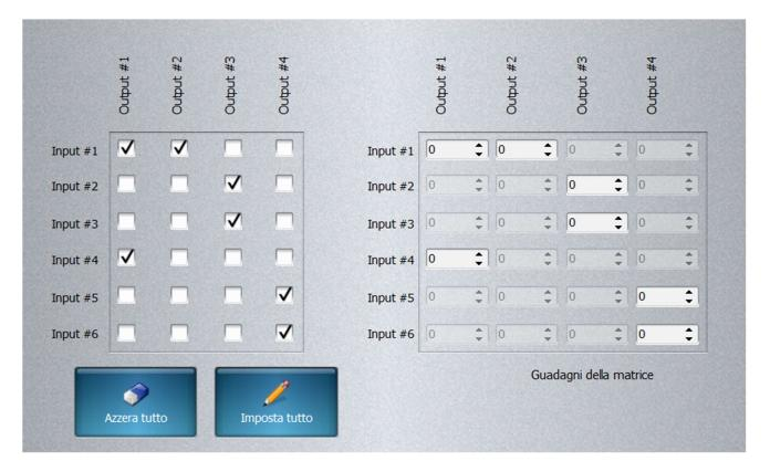
From this section it is possible to direct one or more inputs to one or more outputs by selecting the intersections of the matrix "by putting a check mark".
