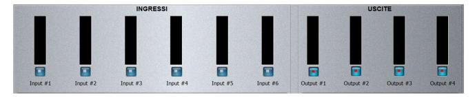
This window is always visible in any work environment you are; it is thus possible to check inputs and output level and enable/disable the muting function.
