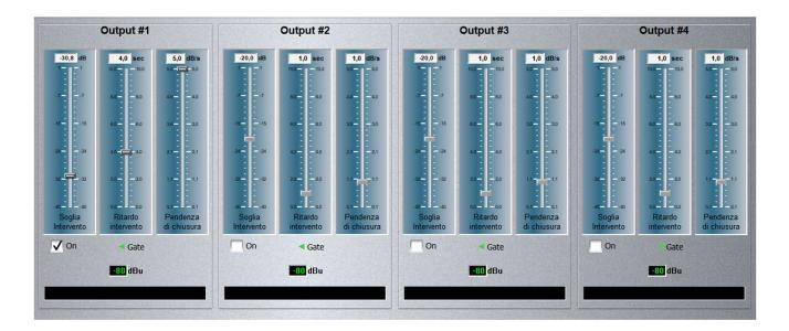
From this section it is possible to enable a noise gate for each output by clicking on "on".
