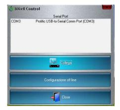
From this window it is possible to select the serial port to connect to the matrix, or perform an off-line configuration, that is, without the device being connected.
