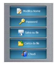
From this section it is possible to change the project name, assign a new password (default \*\*\*\*), save the project on the computer, upload a project from the computer or close the work section.
