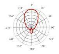
FS 300 is a professional back electret microphone with unidirectional cartridge that gets good effect of hyper-narrow direction and long-distance sounds pick up. It has a hyper-cardiod polar pattern.
